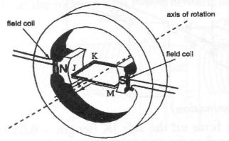
The armature of the motor consists of a rectangular coil with 30 turns. Side JK is 15 cm long and side JM is 10 cm. The magnetic field can be considered to be radial and has a flux density of 0.05 T. A current of 2.09 A is recorded when the motor is running freely.
